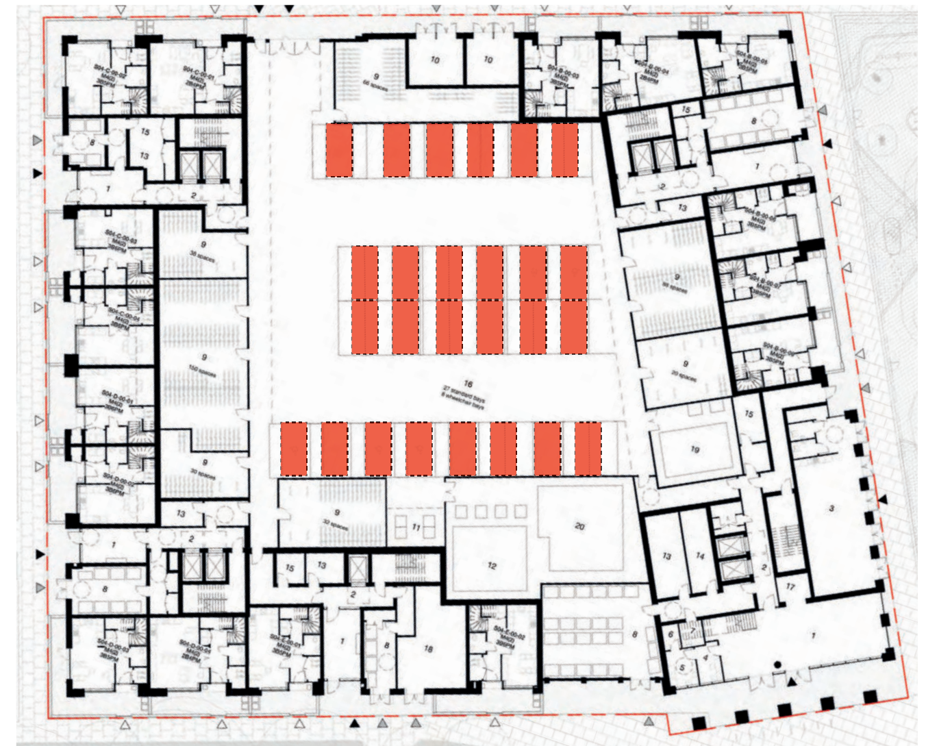
Subplot S04 Proposed Amendments Adapted Adapted to provide 10% Wheelchair Parking Space Provision
