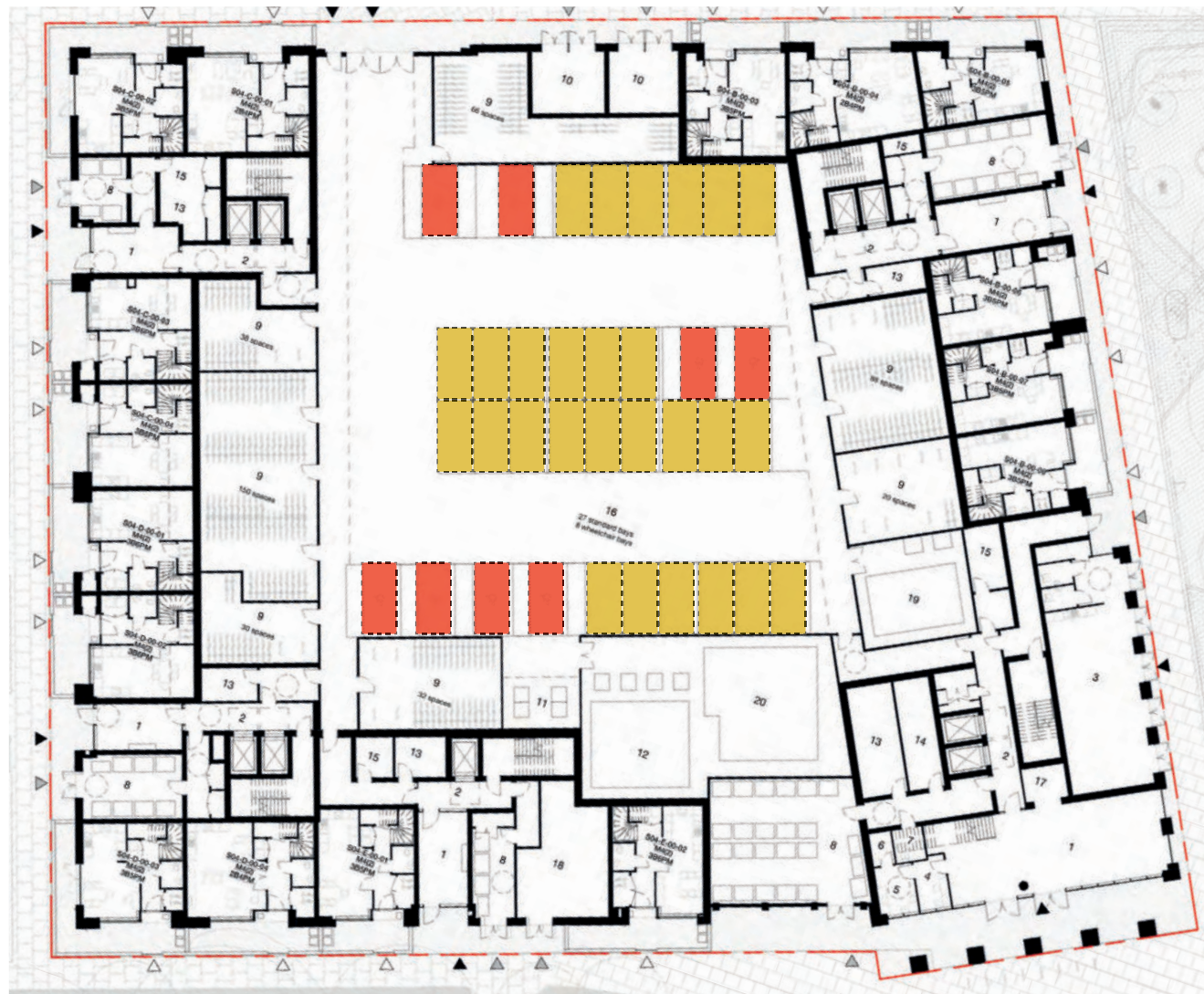
Subplot S04 Proposed Amendments Outlet 3% Wheelchair Parking Space Provision
